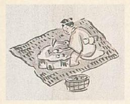
The silver ore is placed on a cornerstone and crushed using a hammer. It is then placed in water and shaken to separate the silver.
