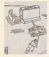
The alloy is placed over a bed of coals and melted. The lead sinks into the coals leaving the silver on top. This process is repeated to increase the purity of the silver.
