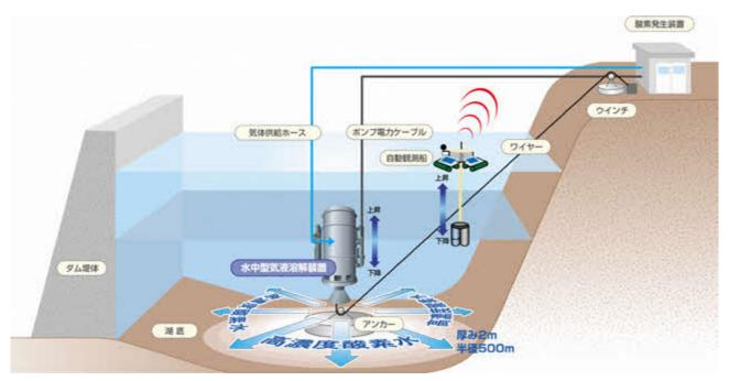
The WEP System is a system designed to solve water quality problems caused by poor oxygen, in which the oxygen level in the water of dams and lakes becomes extremely low.
