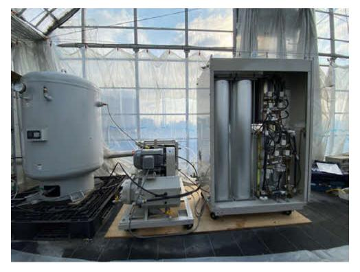
A device to collect and concentrate CO<sub>2</sub> from the atmosphere using natural zeolite produced in Shimane Prefecture
