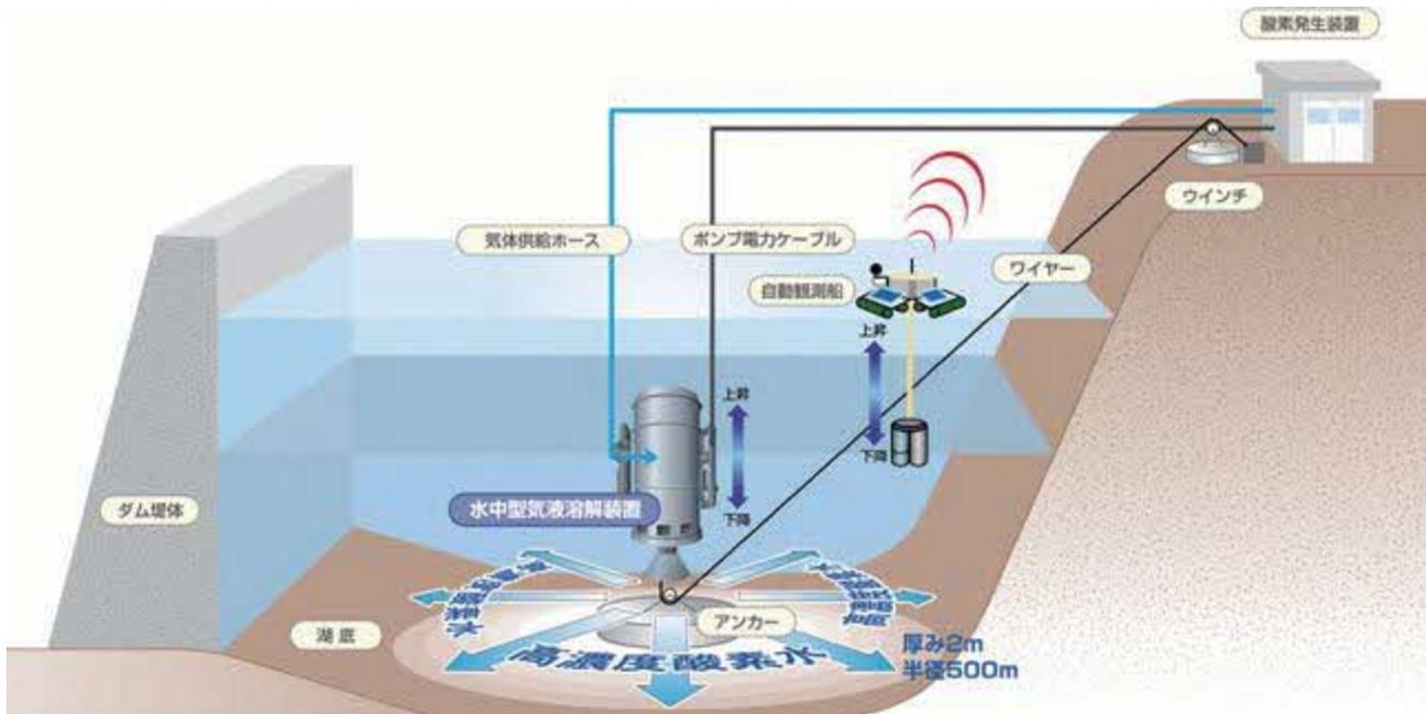
The WEP System is a system designed to solve water quality problems caused by poor oxygen, in which the oxygen level in the water of dams and lakes becomes extremely low.
