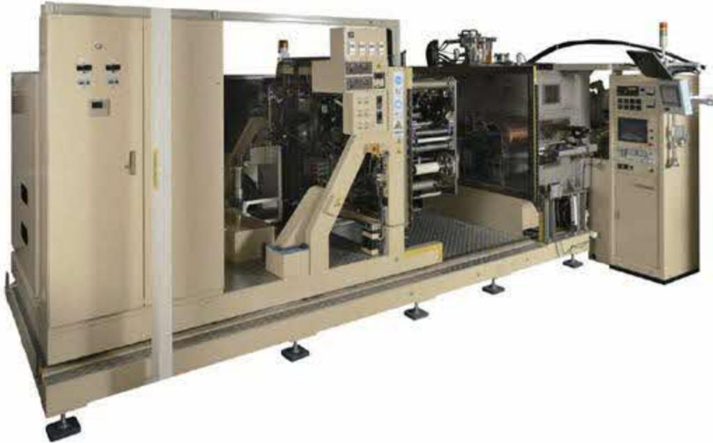
This vacuum deposition device makes it possible to manufacture film capacitor electrodes, lithium battery electrodes and the like by roll to roll. The evaporation sources that can be mounted are resistance heating crucibles, radiant heating crucibles, and E/B sources. A plasma source is also available to improve adhesion between the base material and the deposition layer. It is also capable of handling double-sided deposition.
